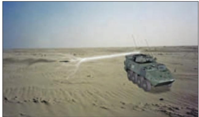
Figure 4. Neutralization of the electronic circuits of an incoming threat by creating an electric conductor.
