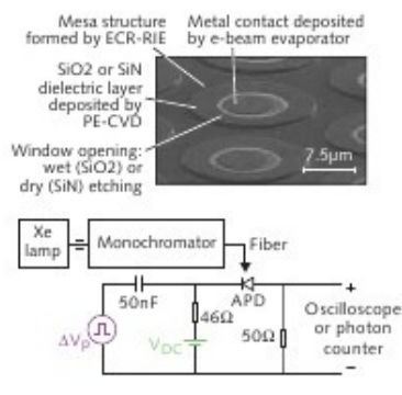
FIGURE 4. A fabricated GaN APD (upper left) uses pulsed quenching circuitry (lower left) for Geiger-mode operation. SPDE varies according to the wavelength of the photon source (right).
