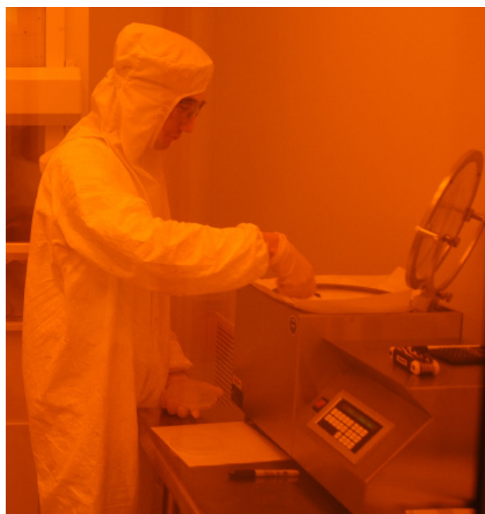
Josh Goldberger, a postdoctoral researcher in the Stupp Group, uses a spin coater to coat a thin film of photoresist onto a silicon wafer in the IBNAM cleanroom core facility. The lighting is yellow/orange to prevent ultraviolet light from prematurely exposing the photoresist, which Goldberger compares to the exposure of undeveloped film in a camera. Photograph used courtesy of Josh Goldberger
